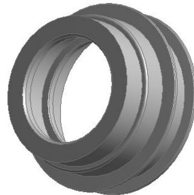
Figure 1 shows a solid 3-D model of bearing support
