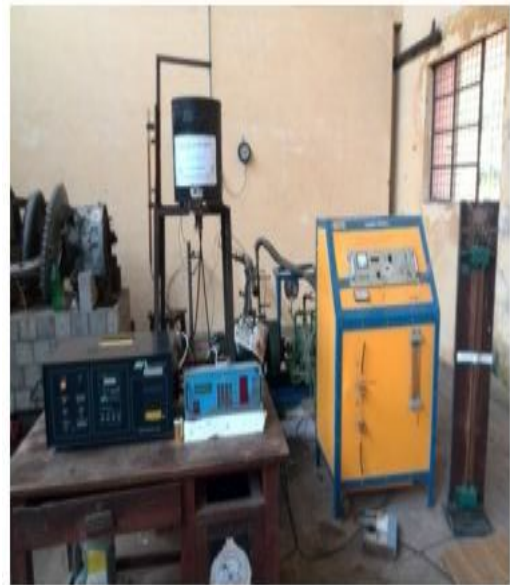
Figure 4. Experimental set up of C.I. Engine
