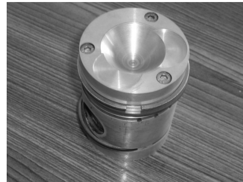
Fig 2: Air-gap insulated Aluminium piston
