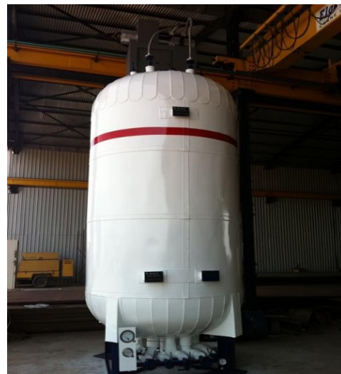
Fig: 1.1 Typical Vertical LPG Storage Vessel Assembly.
