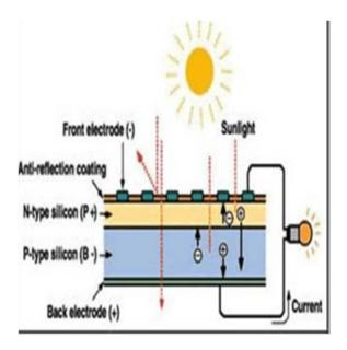
When photons with sufficient energy hit the cell, they cause electrons to move (from N to P only) causing excess electrons in the N-layer and a shortage in the P-layer.
