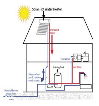
Figure shows a basic schematic of a solar hot water system which is located on the roof of a home. The system depicted is an evacuated tube collector with an active flow circulation and directly uses the work fluid which would be the water.
