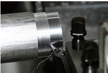
A lathe cutting material from a workpiece.
