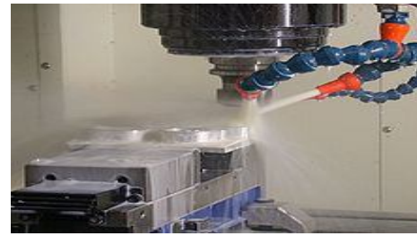
A milling machine in operation, including coolant hoses. Main article: Milling (machining)
