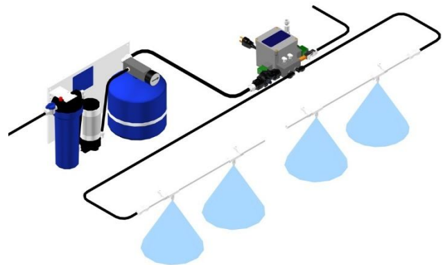
Figure(A) Full Water Misting System
