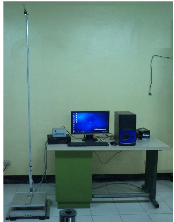
Fig.3- Microcontroller based BMI Calculator with Database and Monitor Display
