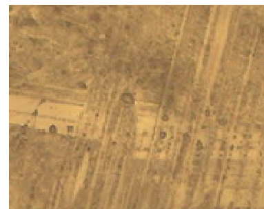
Figure 5. Misalignment of fibres
