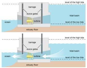
Two current technologies which are used to harness the kinetic energy of tidal flow:
