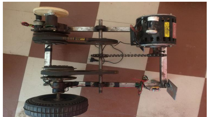
Figure 2: Regenerative clutch model developed – Top view
