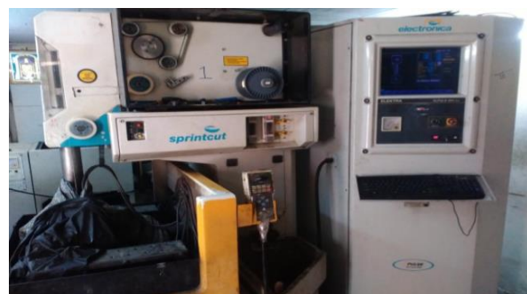
Fig. 1 Wire EDM setup for experimentation
