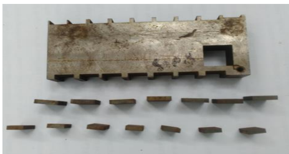
Fig. 2 Machined work piece with cut pieces
