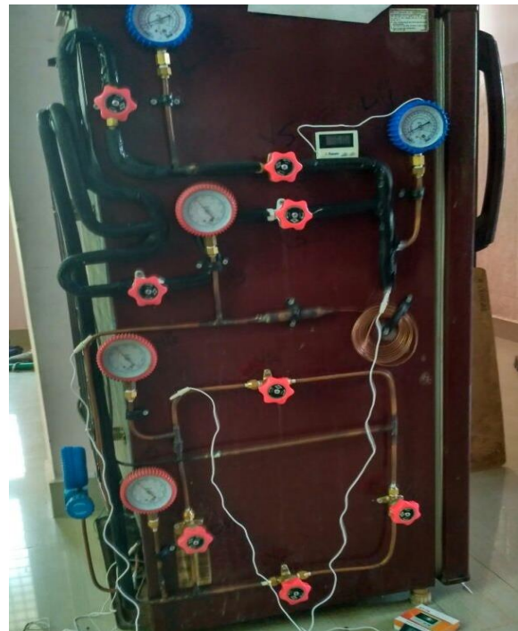
Fig.2.9 Refrigerator with Nozzle at inlet of Evaporator
