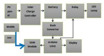
Fig. 1 Block diagram of the system
