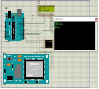
Fig. 6 Proteus simulation of the notice board model
