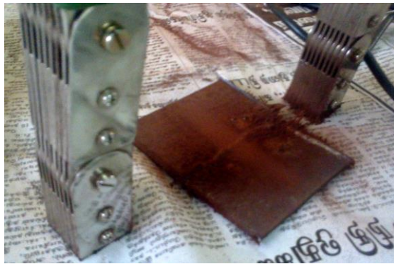
Fig. 5.1. Magnetic particle inspection
