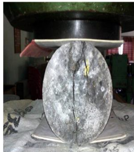
Fig.2 Failure of cylinder under split tension
