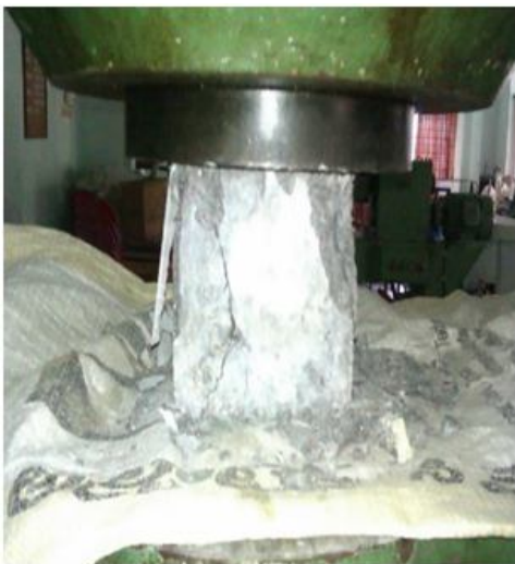
Fig.1 Failure of cube under compression
