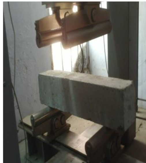
Fig.3 Flexural strength setup
