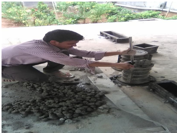
Fig.3 compacting of cylinder
