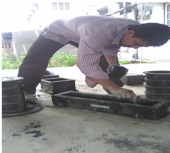
Fig.4 applying oil for beam mould
