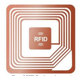
Figure 2:RFID Tag (internal structure)
