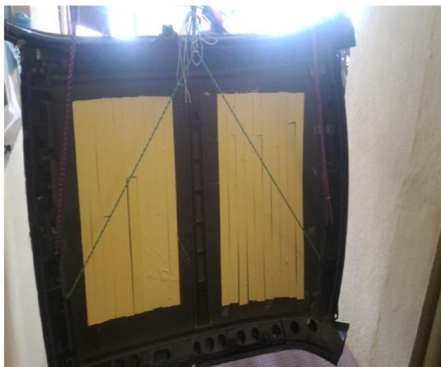
Fig.2. Automotive car floor with damper
