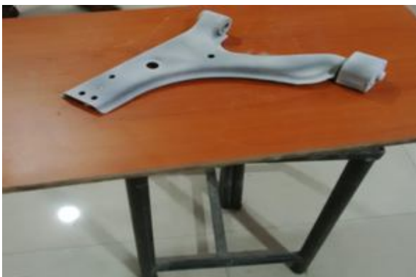
Figure 2: Lower control arm during blue light scanning
