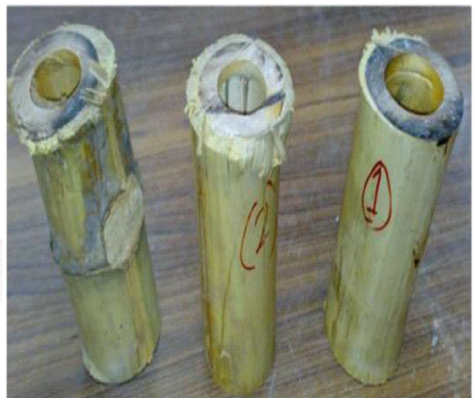
Fig 4.2: Failed bamboo samples in compression test
