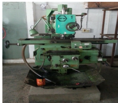
Fig 2: universal milling machine
