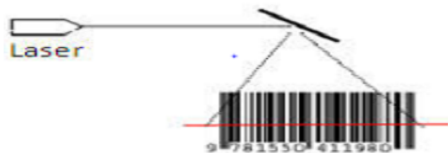
Fig2: Working of Barcode
