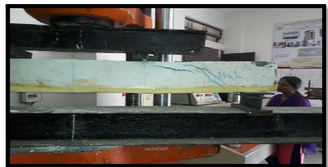
Fig.No.6: Flexural and Shear crack pattern for AFRP strengthened beam.
