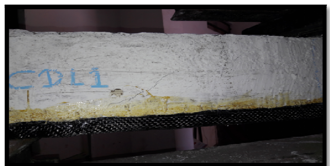
Fig.No.7: Flexural and Shear crack Pattern for CFRP strengthened beam
