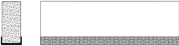
Fig.No.2Applying fiber on beam specimen
