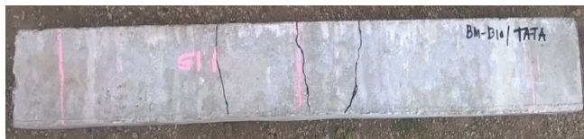
Figure-17. Crack pattern of the failed specimen BM-B10-1-550
