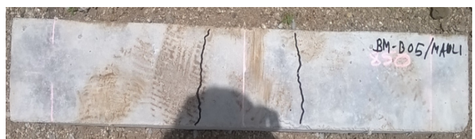
Figure-16. Crack pattern of the failed specimen BM-B05-1-500
