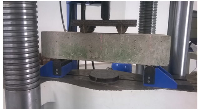
Figure-2. Test set-up for the beam BM-B01-1-550
