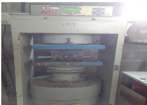
Figure 5 Concrete Specimens Testing
