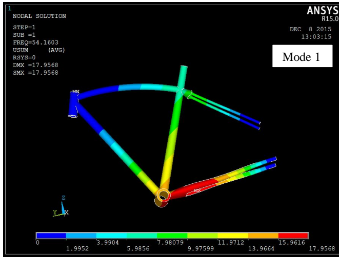
Fig.21 1 st mode frequency of bicycle chassisThe frequency of 1 st mode is 54.16hz.
