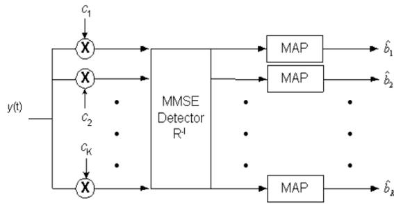
Figure 1: Linear Multiuser Detector Block Diagram
