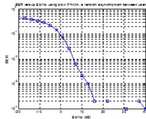
Fig. 4. BER versus SNR for slow FH-MA
