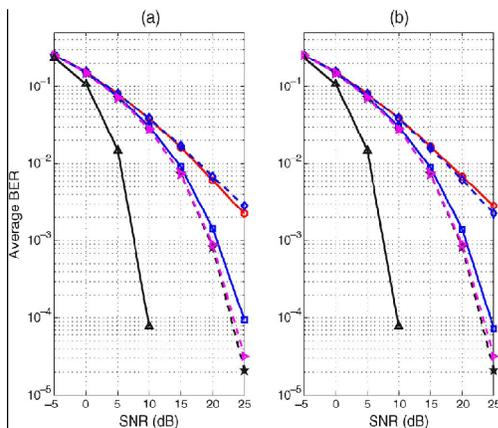
Fig.2. Convergence of BER versus SNR for the S-FT-domain MMSEMUD at K=40 M=8 and N=12
