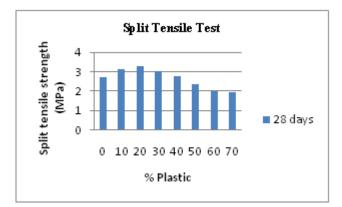
From the graph it can be maximum strength is obtained for the replacement of 10-20% of the plastic replacement.
