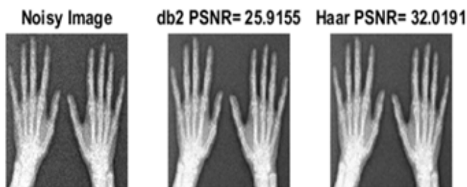
Fig.4: X-Ray image of Hands and PSNR comparison of Base and Proposed method.
