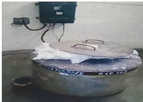
Figure 1 Melting furnace and graphite crucible
