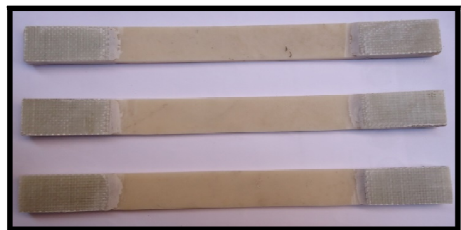
Fig.6.1 specimen before Tensile test
