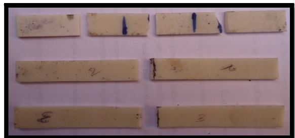
Fig.6.6 specimen after Bending test
