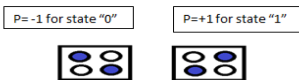
(b) The two different states of a QCA cell.
