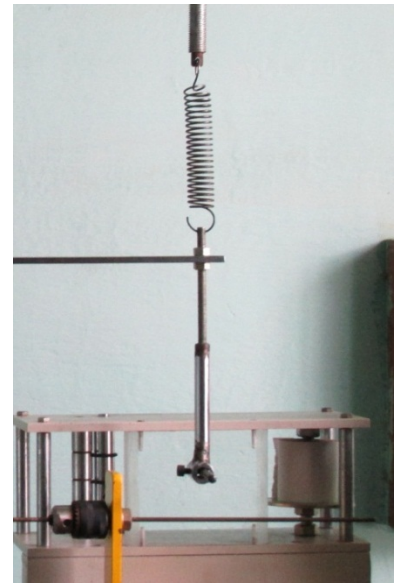
Figure 3.8: Installed straight pencil holder with spring.
