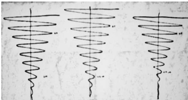
Graph 4.1: Trace obtained from damped torsional vibrations.
