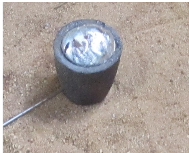
Fig.1.5. The bubble created in the melt through gas injection
