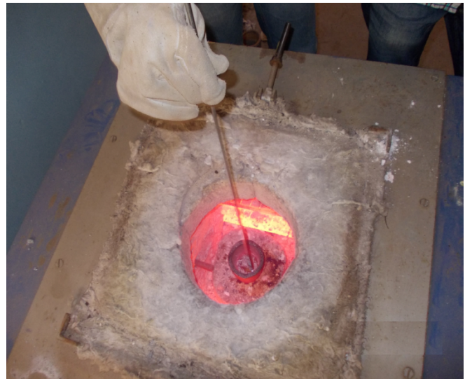
Fig.1.3. Melt stirring using SS pipe 4mm inner diameter
