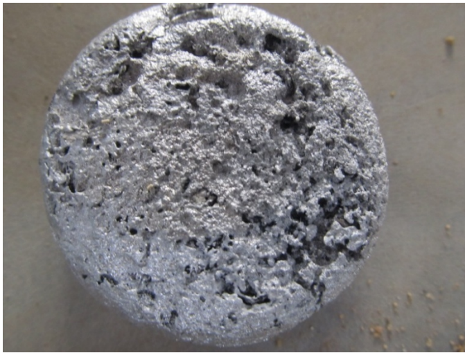
Fig.1.6. The Foam structure obtained by MGI
