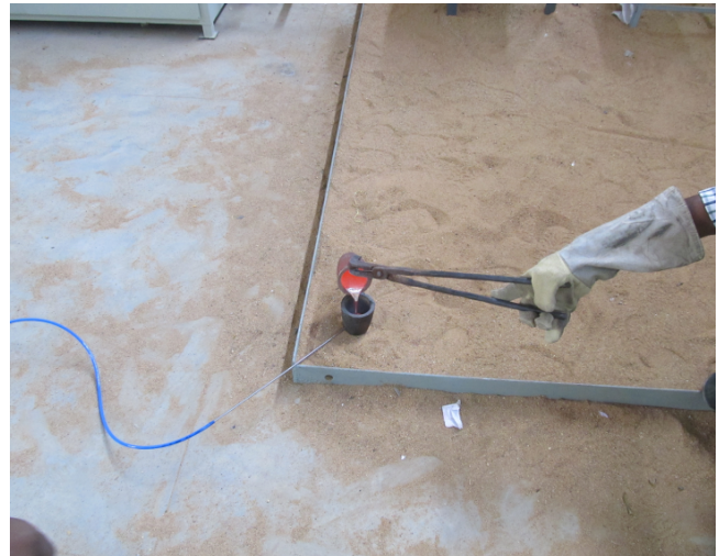
Fig 1.4. Transferring melt into another Crucible
