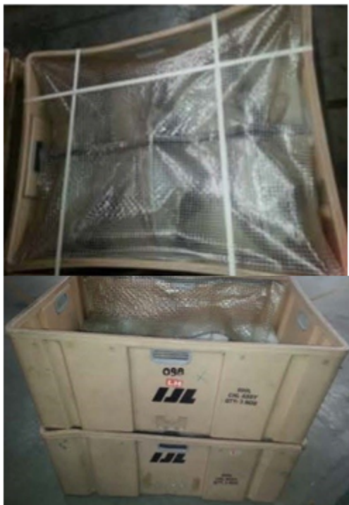
Fig 4: Wall bending and stacking of roto bins
