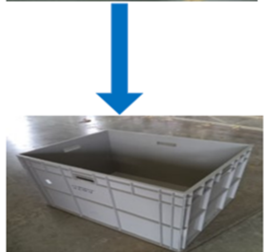
Fig 2: Changing from Roto to Injection bin
