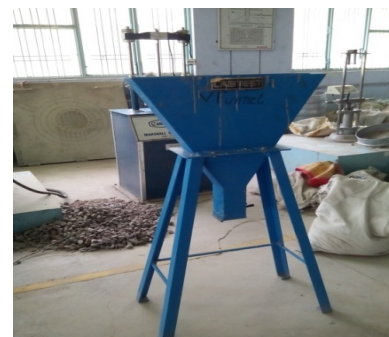
L-Box test and casting specimen V-Funnel Test
