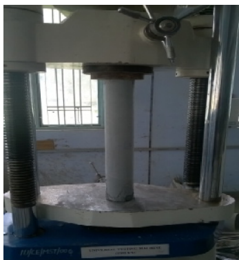
Fig-4 Testing of confined cylinder (UTM)
