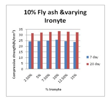
Then we replaced 10% fly ash & varying % of ironyte by weight of cement and we get maximum compressive strength in 10% ironyte and 10% fly ash.
