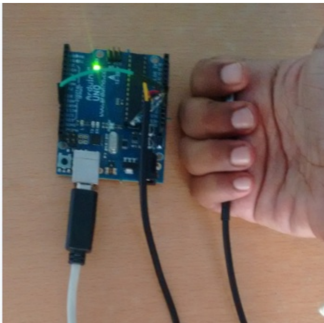
Figure 1 Hardware setup of Temperature sensor.
