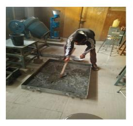
Make cement slurry as stated above proportion and put R.A. in to it for 24 hours. After 24 hours R.A. get out from the slurry and make them totally dry and then used in the concrete.
