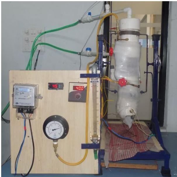
Image 1. Experimental set up of CLPHPs with insulation
