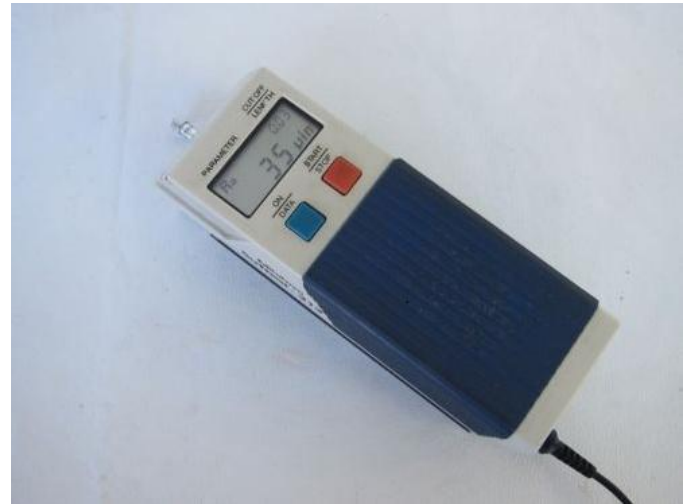
Fig. 3: Profilometer for Roughness Measurement
