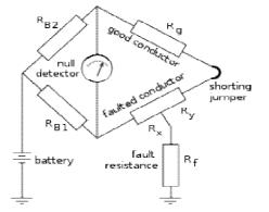
**Murray loop bridge** is a bridge circuit used for locating faults in underground or underwater cables. It has been used for more than 100 years.
