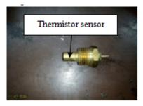
The above picture shows a temperature sending unit. A thermistor is placed inside this sender unit. The thermistor measures the instantaneous change in the temperature of the coolant by changing its resistance. As shown in the picture, the part of the sending unit where the thermistor lies is in contact with the coolant inside the engine. Thermistor has high resolution and greater precision compared to RTD and Thermocouple. Therefore it is implemented in the temperature sending unit.[1]
