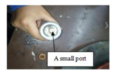
The above picture shows a small port present on the front side of the pressure gauge sending unit. This portion of the sending unit is in contact with the oil inside the engine. Through this port, oil pressure enters in the sending unit.(3)
