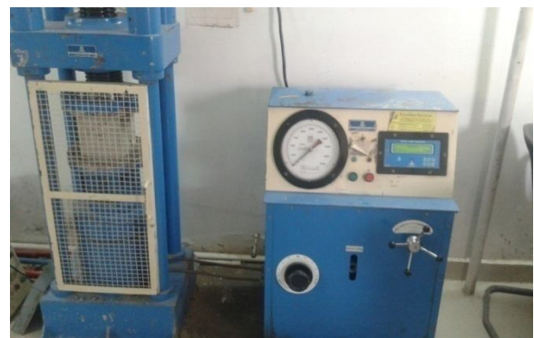
Fig-3 Testing Of Cube
