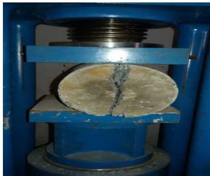
Figure 4.2 Indirect Tensile Test Machine
