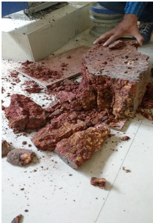
Fig 7: Broken Laterite block.
