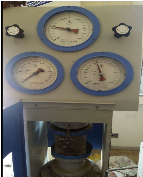
Fig 6: testing of cube specimen
