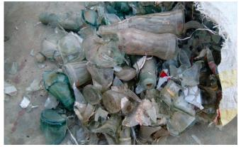
composition and the physical properties of glass which are similar to that of sand and cement Crushed waste glass bottles are in environmental problem, but also provide an available resource for potential use in production of cement, mortar, and concrete by partially replacing coarse and fine natural aggregates.
