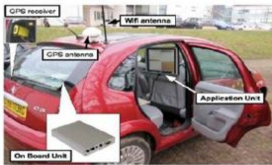
Fig.2 Example of OBU, AU [11]
